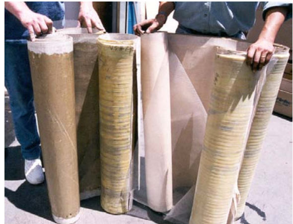
Figure 2: A membrane “autopsy” clearly shows the difference between fouled (left) and unfouled (right) membranes.
